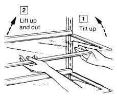
To remove shelves: Tilt shelf up at front, then lift it up and out of tracks on rear wall of refrigerator,
